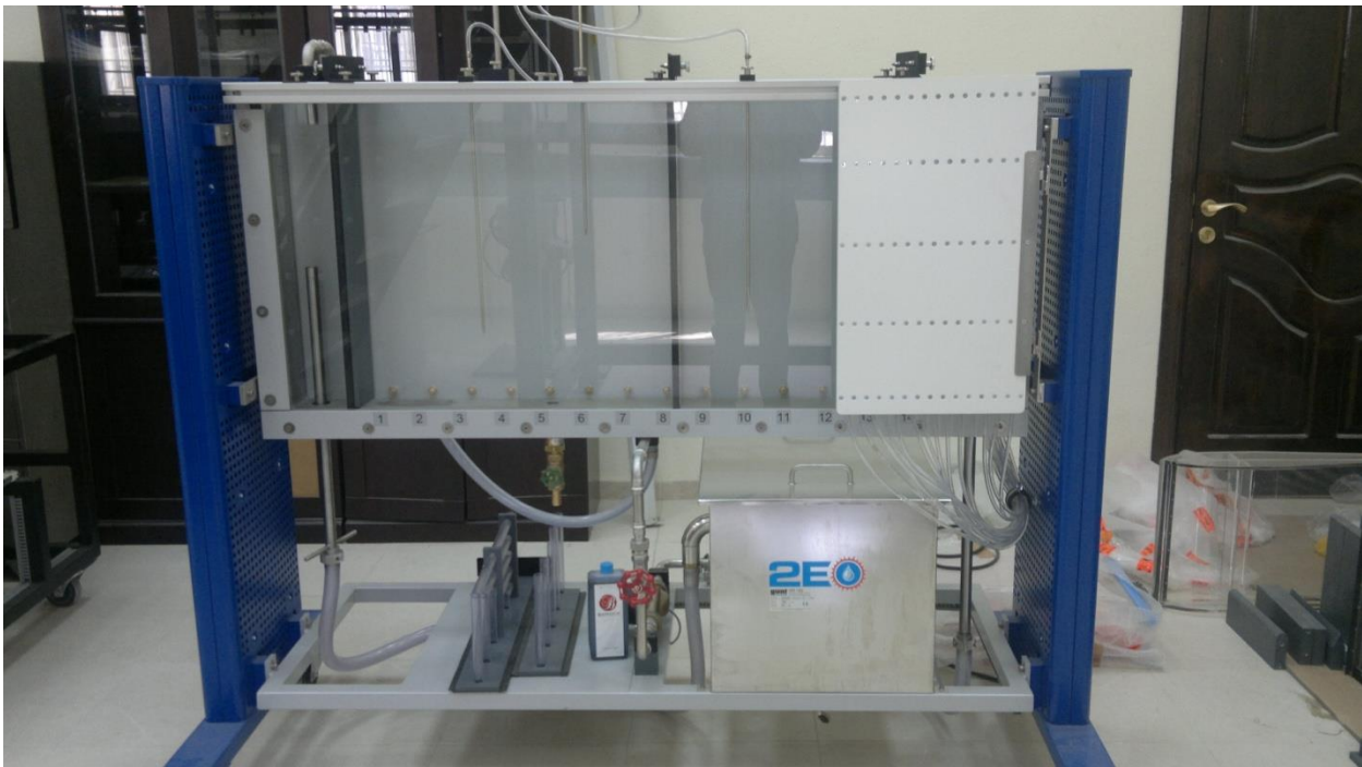
Figure (3): Drainage and Seepage Tank
