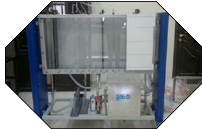
Drainage and Seepage Tank (HM169).
