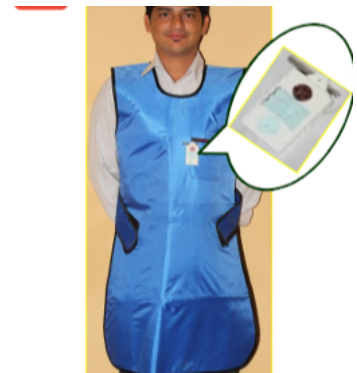
Figure 6 incorrect position TLD below apron
