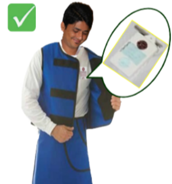
Figure 5 correct position TLD below apron
